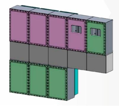
Drawing 1: Typical modular dual redundant battery charger
